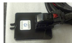
Transmission Control Unit Connection
