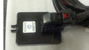
Transmission Control Unit Connection
